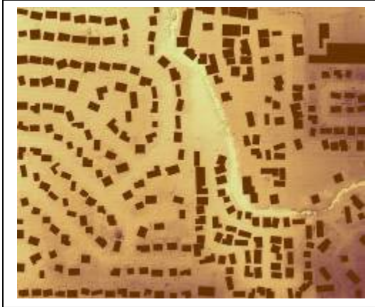
The image on the left shows the extraction of building footprints from the LIDAR data. The image on the right shows the 3D buildings on top of the hill shaded terrain model.
